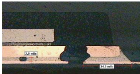
50% paste coverage, plugged via, 2.9 mil standoff
