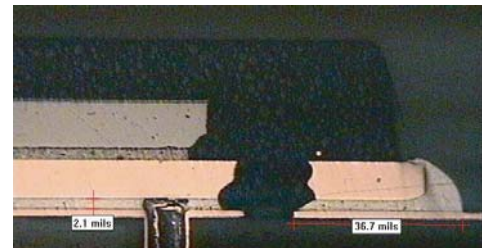
81% paste coverage, encroached via, 2.1 mil standoff
