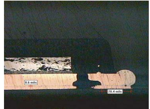
37% paste coverage, encroached via, 0.6 mil standoff
