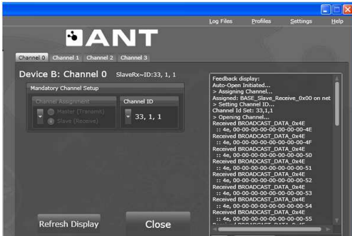
Figure 3 – 3. Slave Channel Configuration
