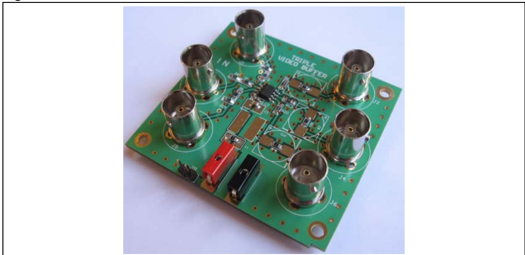
Figure 1. TSH173 evaluation board
