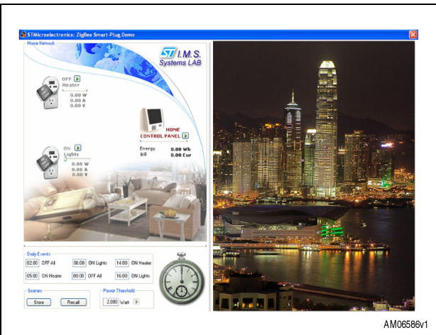
Figure 5. PC GUIs available to show ZigBee smartplug network features: internal demo GUI
