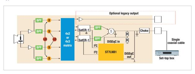
ST7LNB1 is perfectly suited to control the ST satellite channel router, SaTCR, offering a single cable solution and excellent cost-saving advantages in multi receivers for single or collective home environments.
