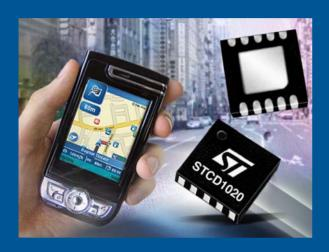
The STCD1020, STCD1030 and STCD1040 are 2-, 3- or 4-channel output, unity-gain clock distribution circuits that are ideal for providing a common frequency clock to multi-mode mobile RF applications. They can also be used in mobile phones as a clock reference for baseband peripheral applications such as WLAN, Bluetooth, GPS and FM radio.
