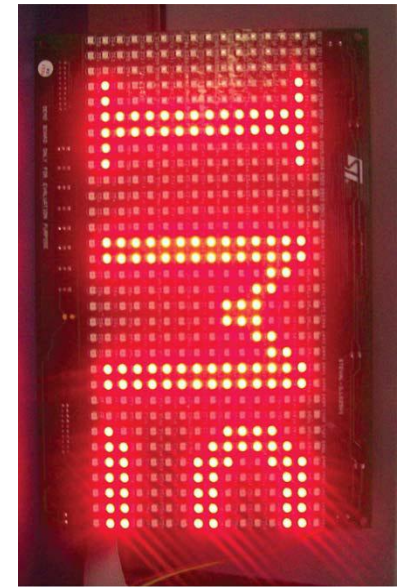
STEVAL-ILL025V1 shows capability of STP16DP05 in driving matrix LED display panel
