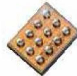
CSP 1.4 x 1.8 mm 12 bumps 0.4 mm pitch
