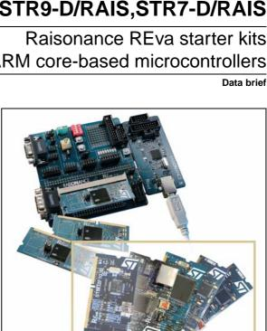
evaluation board, microcontrollers, embedded RLink JTAG in-circuit debugger/programmer and **Raisonance Integrated Development Environment** (RIDE).
