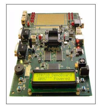
The STR710-EVAL integrates a 2x16 LCD, LEDs, UART, CAN and USB interfaces, piezo buzzer and test buttons in a versatile stand-alone test platform.
