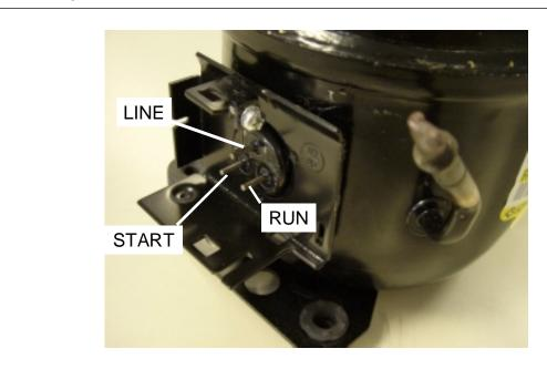
Often, compressor motors are used with a starter that includes a thermal protection against excessively high currents or overheating. This protection is called a "klixon", and is shown in Figure 7. When you are using the THERM01EVAL board its better to keep this starter, in order to let the klixon work. In this case, the motor connections can still be accessible, this depends on the starter model, as shown in Figure 7.
