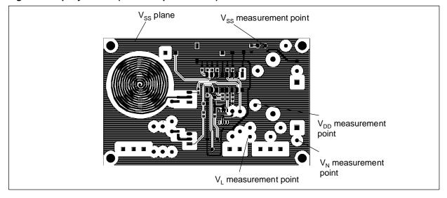
Figure 4. Bottom layer view (from component side)
