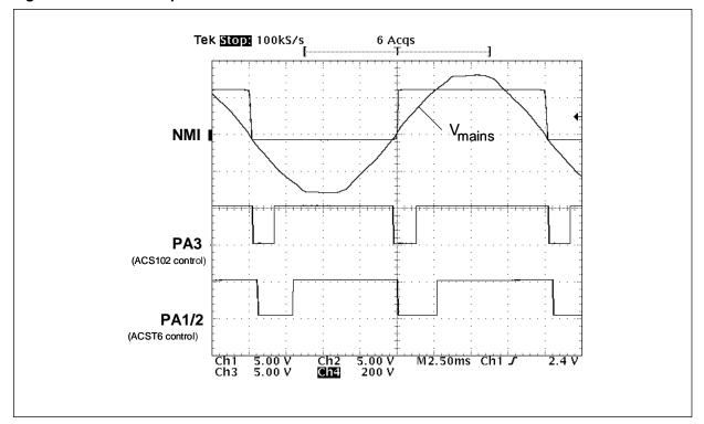
Figure 2. Gate current pulses
