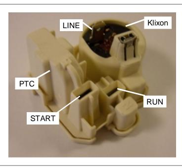
If you want to keep the PTC acting inside the starter, then the RUN pin must not be connected to the "RUN" connector of the THERM01EVAL board.
