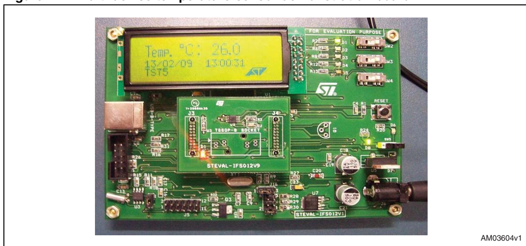
Figure 1. Multi-device temperature-sensor demonstration board
