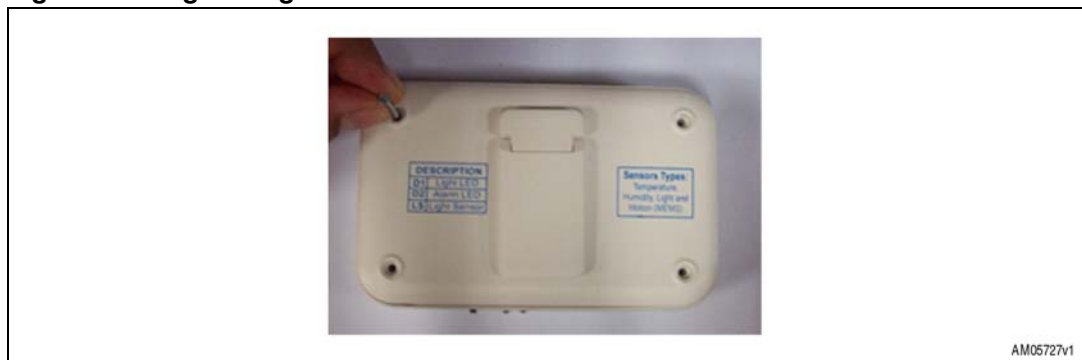
Figure 43. Tightening the screws
