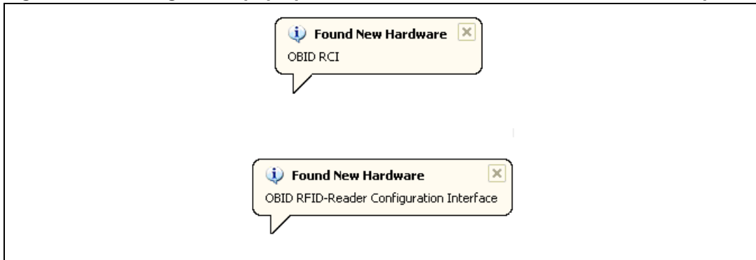
Figure 9. Messages that pop up when the RF reader is connected to the computer
