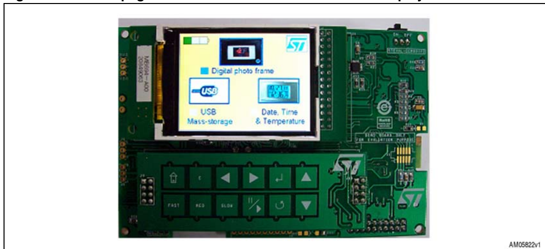
Figure 4. Home page with DPF icon selected on the TFT display
