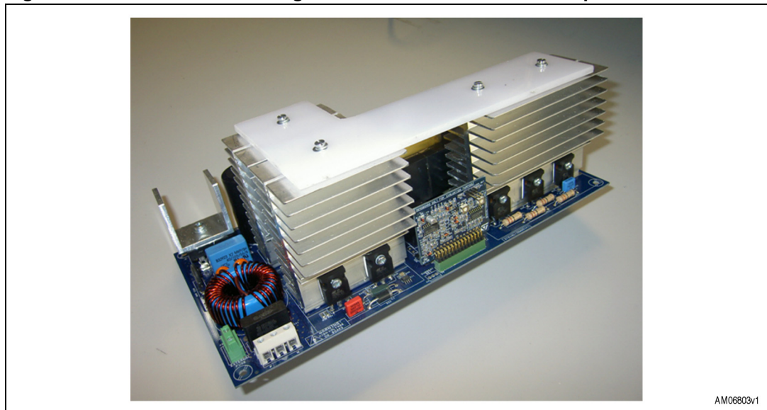
Figure 2. 2.5 kW/135 A welding machine STEVAL-ISW001V1 top view
