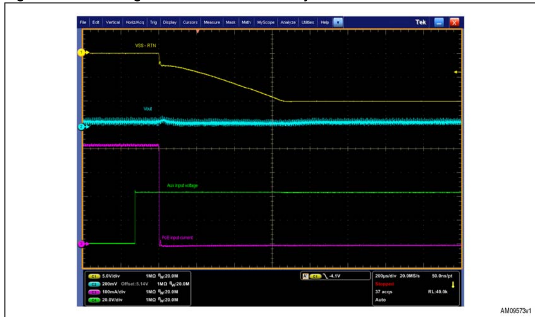
Figure 18. Switching between PoE and auxiliary source
