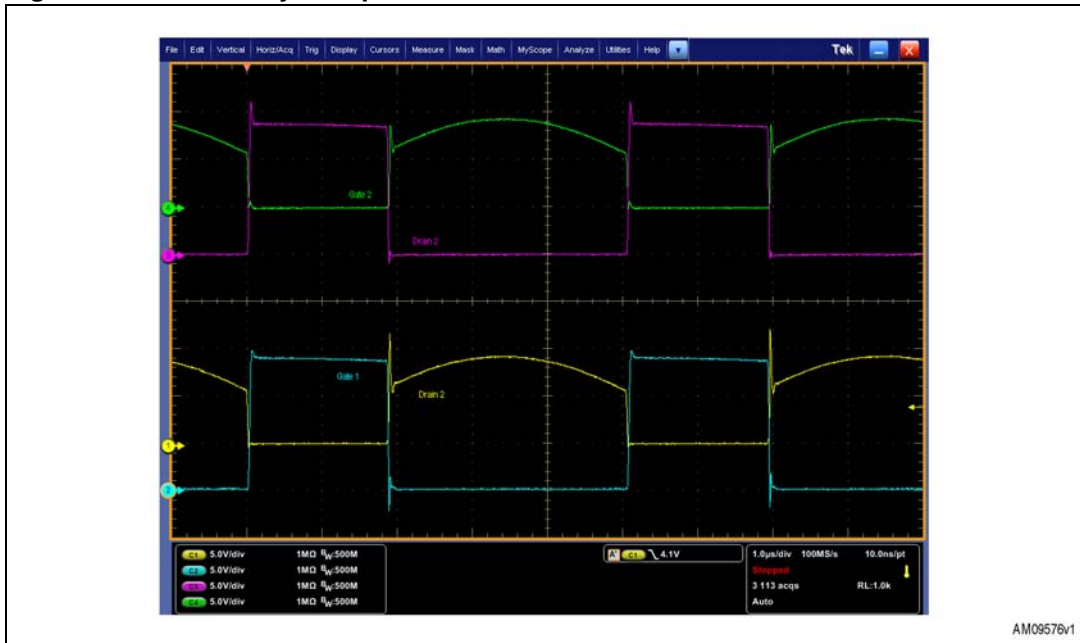
Figure 22. Secondary side power MOSFET waveforms at 4 A load
