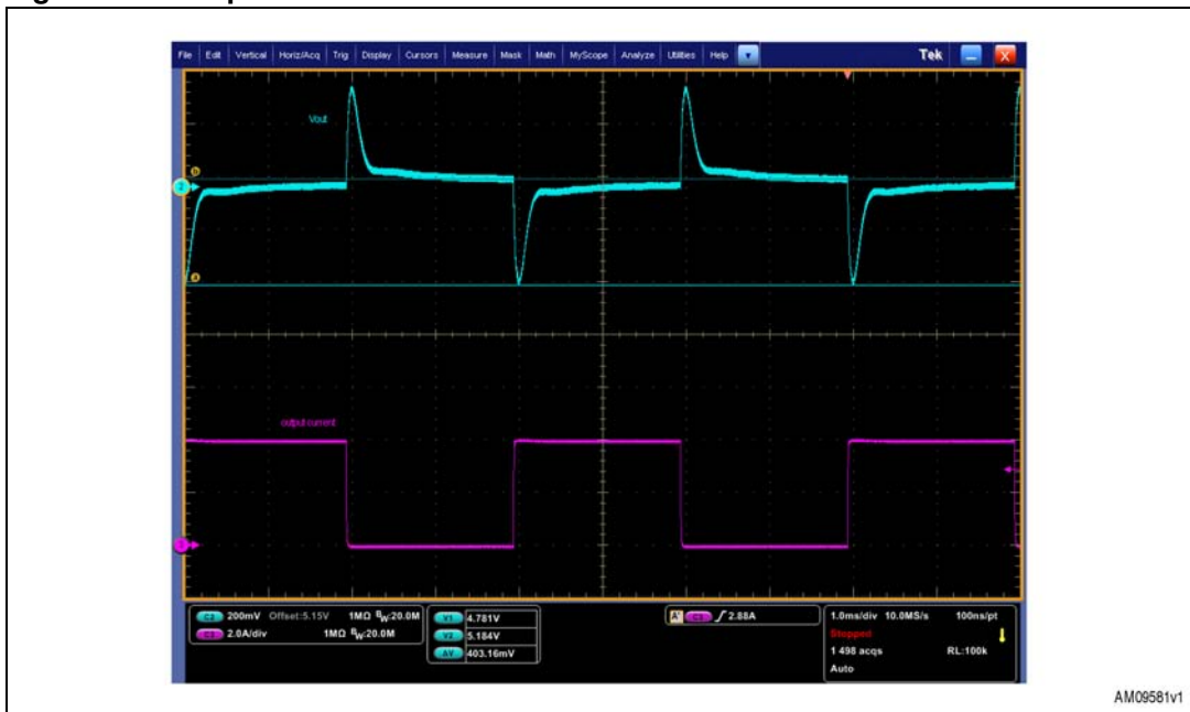
Figure 26. Response of the converter to a 0 A - 4 A load transient
