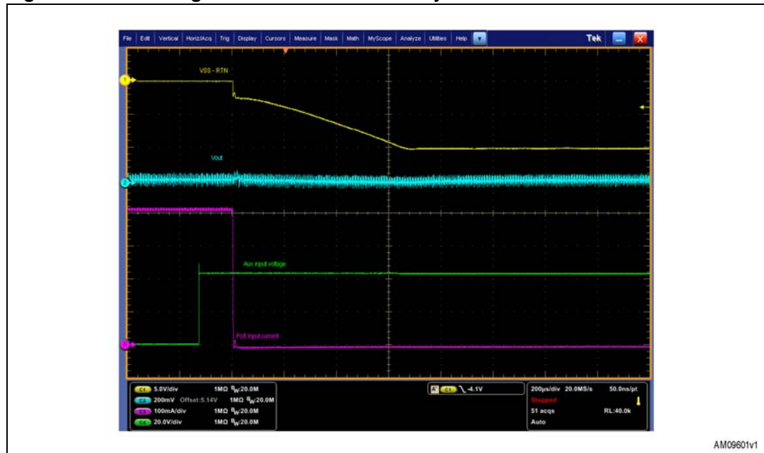
Figure 18. Switching between PoE and auxiliary source
