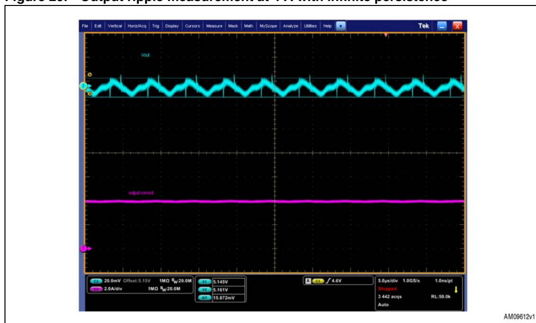
Figure 29. Output ripple measurement at 4 A with infinite persistence
