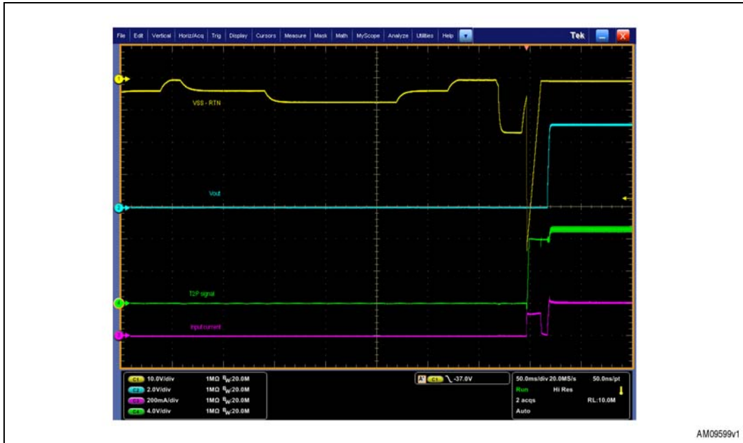
Figure 16. Startup from an IEEE 802.3af injector with 2 A load
