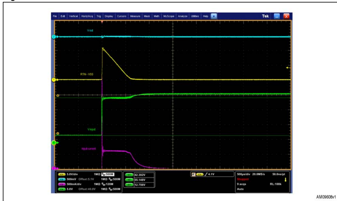
Figure 25. Effect of a 12 V line transient on the converter at 0 A load
