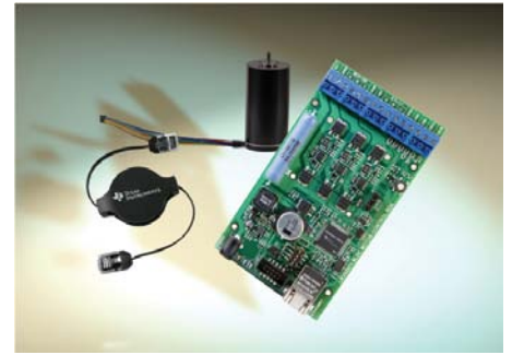
▲ Stellaris RDK-BLDC brushless DC motor control with connectivity reference design kit
