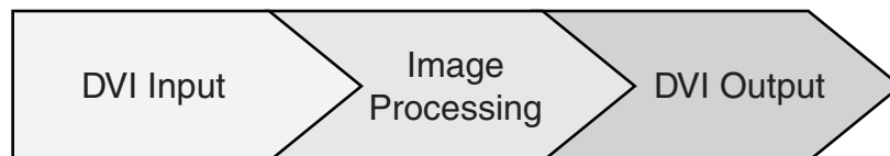
Figure 4-2: DVI Pass-Through Pipeline
