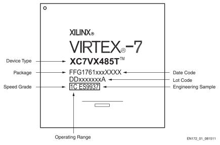
Figure 1: Example Device Top Mark
