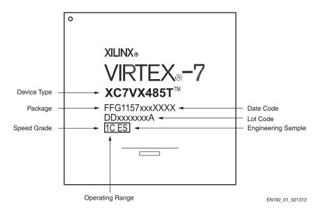
Figure 1: Example Device Top Mark
