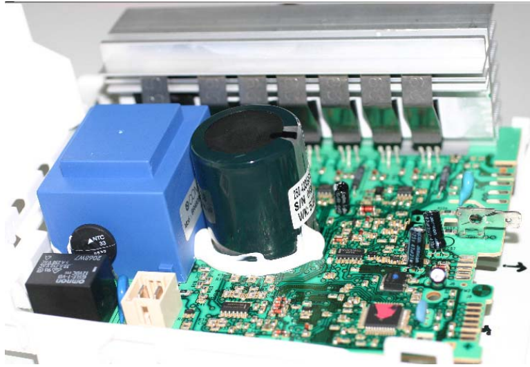
Figure 16: Commercial board with TO-220 FullPAK + clips
