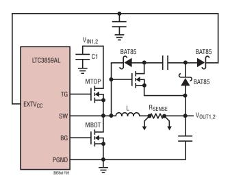
Figure 9. Capacitive Charge Pump for  $\mathsf{EXTV}_\mathsf{CC}$
