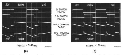
Figure 1. Input Waveforms Comparing Single-Phase (a) and 2-Phase (b) Operation for Dual Switching Regulators Converting 12V to 5V and 3.3V at 3A Each. The Reduced Input Ripple with the 2-Phase Regulator Allows Less Expensive Input Capacitors, Reduces Shielding Requirements for EMI and Improves Efficiency
