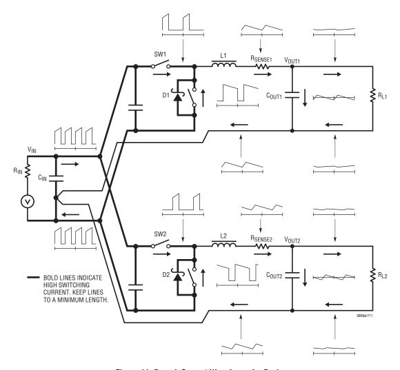
Figure 11. Branch Current Waveforms for Bucks
