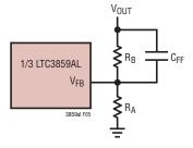
Figure 5. Setting Output Voltage
