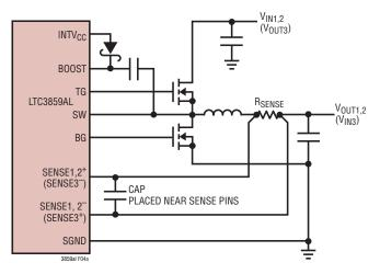
4a. Using a Resistor to Sense Current
