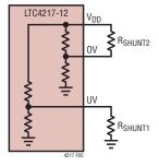
Figure 5. Adjusting LTC4217-12 Thresholds
