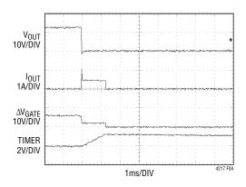
Figure 4. Short-Circuit Waveform
