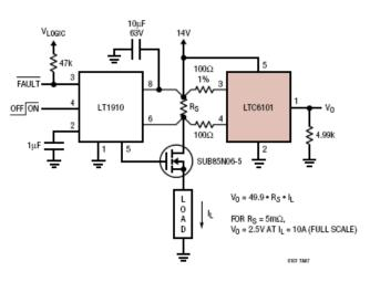
The LT1910 is a dedicated high side MOSFET driver with built in protection features. It provides the gate drive for a power switch from standard logic voltage levels. It provides shorted load protection by monitoring the current flow to through the switch. Adding an LTC6101 to the same circuit, sharing the same current sense resistor, provides a linear voltage signal proportional to the load current for additional intelligent control.
