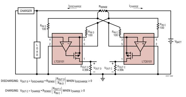
In this circuit the outputs are enabled by the direction of current flow. The battery current when either charging or discharging enables only one of the outputs. For example when charging, the  $V_{OUT}$  D signal goes low since the output MOSFET of that LTC6101 turns completely off
