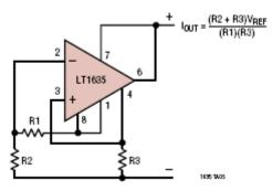
The LT1635 combines an op amp with a 200mV reference. Scaling this reference voltage to a potential across resistor R3 forces a controlled amount of current to flow from the +terminal to the –terminal. Power is taken from the loop.
