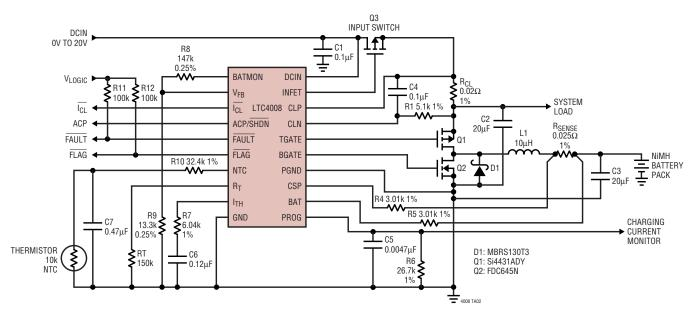
The LTC4008 is a complete NiMH battery pack controller. It provides automatic switchover to battery power when the external DC power source is removed. When power is connected the battery pack is always kept charged and ready for duty.
