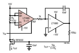
The LT1995 amplifies the sense resistor drop by 5V/V and subtracts that from  $V_{IN}$ , providing an error signal to an LT1880 integrator. The integrated error drives the PMOSFET as required to deliver the commanded current.
