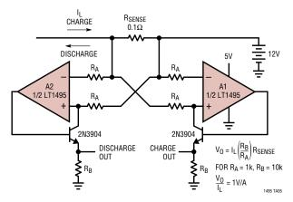
One LT1495 dual op-amp package can be used to establish separate charge and discharge current monitoring outputs. The LT1495 features Over-the-Top operation allowing the battery potential to be as high as 36V with only a 5V amplifier supply voltage.
