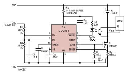
This load protecting circuit employs low-side current sensing. The N-MOSFET is controlled to soft-start the load (current ramping) or to disconnect the load in the event of supply or load faults. An internal shunt regulator establishes a local operating voltage.
