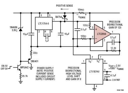
Using a very precise zero-drift amplifier as a pre-amp allows for the use of a very small sense resistor in a high voltage supply line. A floating power supply regulates the voltage across the pre-amplifier on any voltage rail up to the 60V limit of the LT1787HV circuit. Overall gain of this circuit is 1000. A 1mA change in current in either direction through the  $10m\Omega$  sense resistor will produce a 10mV change in the output voltage.
