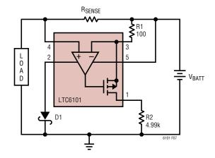
The LTC6101 is not protected internally from external reversal of supply polarity. To prevent damage that may occur during this condition, a Schottky diode should be added in series with V<sup>-</sup>. This will limit the reverse current through the LTC6101. Note that this diode will limit the low voltage performance of the LTC6101 by effectively reducing the supply voltage to the part by V<sub>D</sub>.
