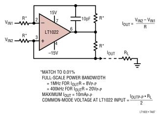
This is a variation on the Howland configuration, where load current actually passes through a feedback resistor as an implicit sense resistance. Since the effective sense resistance is relatively large, this topology is appropriate for producing small controlled currents.
