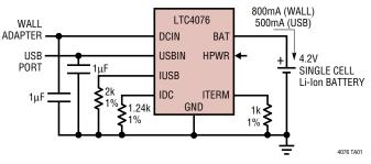
Just a few external components are required for this single Li-Ion cell charger. Power for the charger can come from a wall adapter or a computer's USB port.
