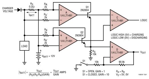
Op-amp sections A & B form classical high-side sense circuits in conjunction with Q1 & Q2 respectively. Each section handles a different polarity of battery current flow and delivers metered current to load resistor  $R_G$ . Section C operates as a comparator to provide a logic signal indi-
