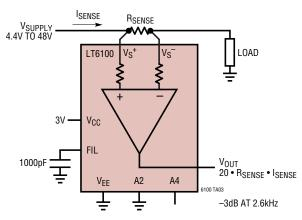
The LT6100 has pin strap connections to establish a variety of accurate gain settings without using external components. For this circuit grounding A2 and leaving A4 open set a gain of 20. Adding one external capacitor to the FIL pin creates a low-pass filter in the signal path. A capacitor of 1000pF as shown sets a filter corner frequency of 2.6KHz.
