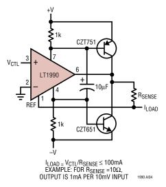
This is a classical Howland bidirectional current source implemented with an LT1990 integrated difference amplifier. The op amp circuit servos to match the RSENSE voltage drop to the input command VCTL. When the load current exceeds about 0.7mA in either direction, one of the boost transistors will start conducting to provide the additional commanded current.
