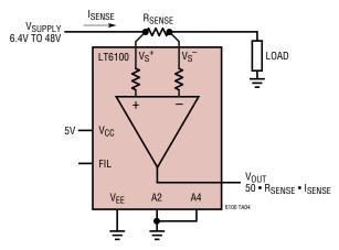
The LT6100 is configured for a gain of 50 by grounding both A2 and A4. This is one of the simplest current sensing amplifier circuits where only a sense resistor is required.
