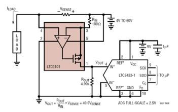
The LTC2433-1 can accurately digitize signal with source impedances up to  $5k\Omega$ . This LTC6101 current sense circuit uses a  $4.99k\Omega$  output resistance to meet this requirement, thus no additional buffering is necessary.
