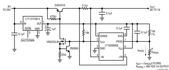
The current output can be controlled by a variable resistor (R<sub>PBOG</sub>) connected from the PROG pin to ground on the LT1620. The LT1121 is a low-dropout regulator that keeps the voltage constant for the LT1620. Applying a
