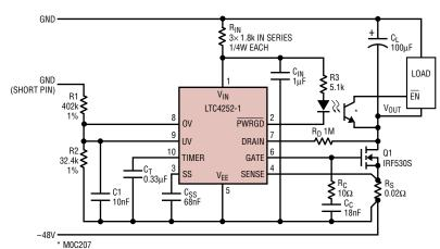
This load protecting circuit employs low-side current sensing. The N-MOSFET is controlled to soft-start the load (current ramping) or to disconnect the load in the
