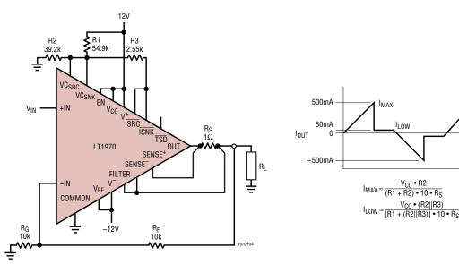
The LT1970 provides current detection and limiting features built-in. In this circuit, the logic flags that are produced in a current-limiting event are connected in a feedback arrangement that in turn reduces the current limit command to a lower level. When the load condition permits the current to drop below the limiting level, then the flags clear and full current drive capability is restored automatically.
