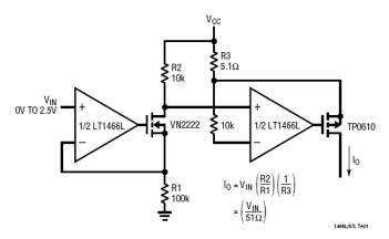
A basic high-side current source is implemented at the output, while an input translation amplifier section provides for flexible input scaling. A Rail-to-Rail input capability is required to have both amplifiers in one package, since the input stage has common-mode near ground and the second section operates near  $V_{CC}$ .
