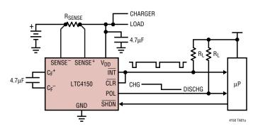
The LTC4150 is a micropower high-side sense circuit that includes a V/F function. Voltage across the sense resistor is cyclically integrated and reset to provide digital transitions that represent charge flow to or from the battery. A polarity bit indicates the direction of the current. Supply potential for the LTC4150 is 2.7V to 8.5V. In the free-running mode (as shown, with CLR & INT connected together) the pulses are approximately  $1\mu$ s wide and around 1Hz full-scale.
