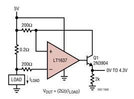
This circuit uses generic devices to assemble a function similar to an LTC6101. A Rail-to-Rail Input type op amp is required since input voltages are right at the upper rail. The circuit shown here is capable of monitoring up to 44V applications. Besides the complication of extra parts, the  $V_{OS}$  performance of op amps at the supply is generally not factory trimmed, thus less accurate than other solutions. The finite current gain of the bipolar transistor is a small source of gain error.
