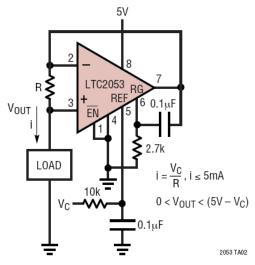
The ultra-precise LTC2053 instrumentation amplifier is configured to servo the voltage drop on sense resistor R to match the command  $V_C$ . The LTC2053 output capability limits this basic configuration to low current applications.
