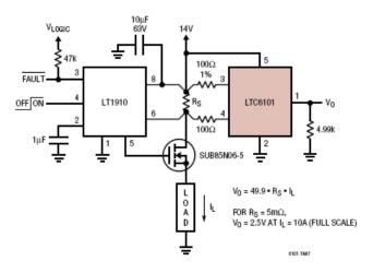
The LT1910 is a dedicated high side MOSFET driver with built in protection features. It provides the gate drive for a power switch from standard logic voltage levels. It provides shorted load protection by monitoring the current flow to through the switch. Adding an LTC6101 to the same circuit, sharing the same current sense resistor, provides a linear voltage signal proportional to the load current for additional intelligent control.
