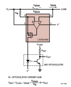
The HV version of the LTC6101 can operate with a total supply voltage of 105V. Current flow in high supply voltage rails can be monitored directly or in an isolated fashion as shown in this circuit. The gain of the circuit and the level of output current from the LTC6101 depends on the particular opto-isolator used.
