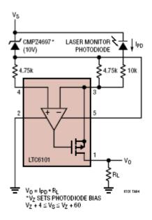
Current through a photodiode with a large reverse bias potential is converted to a ground referenced output voltage directly through an LTC6101. The supply rail can be as high as 70V. Gain of the I to V conversion, the transimpedance, is set by the selection of resistor  $R_L$ .
