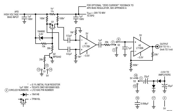
Lock-In Amplifier Technique Permits 1% Accurate APD Current Measurement Over 100nA to 1mA Range.
