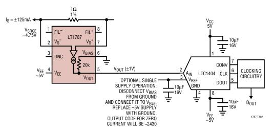
In this circuit, split supply operation is used on both the LT1787 and LT1404 to provide a symmetric bidirectional measurement. In the single-supply case, where the
