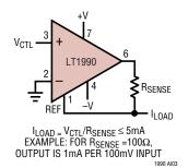
The LT1990 is a differential amplifier with integrated precision resistors. The circuit shown is the classic Howland current source, implemented by simply adding a sense resistor.
