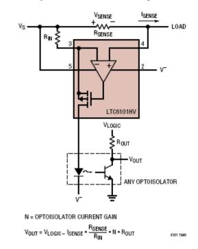
The HV version of the LTC6101 can operate with a total supply voltage of 105V. Current flow in high supply voltage rails can be monitored directly or in an isolated fashion as shown in this circuit. The gain of the circuit and the level of output current from the LTC6101 depends on the particular opto-isolator used.
