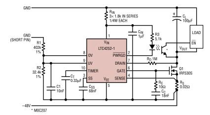
This load protecting circuit employs low-side current sensing. The N-MOSFET is controlled to soft-start the load (current ramping) or to disconnect the load in the event of supply or load faults. An internal shunt regulator establishes a local operating voltage.
