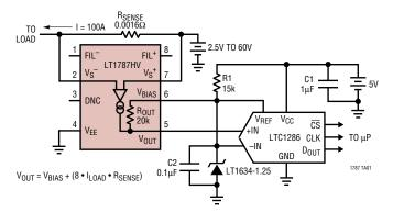
While the LT1787 is able to provide a bidirectional output, in this application the economical LTC1286 is used to digitize a unidirectional measurement. The LT1787 has a nominal gain of eight, providing a 1.25V full-scale output at approximately 100A of load current.
