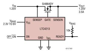
The LTC4213 provides protection and automatic circuit breaker action by sensing Drain-to-Source voltage-drop across the NMOSFET. The sense inputs have a Rail-to-Rail common mode range, so the circuit breaker can protect bus voltages from 0V up to 6V. Logic signals flag a trip condition (with the READY output signal) and reinitialize the breaker (using the ON input). The ON input may also be used as a command in a "smart switch" application.
