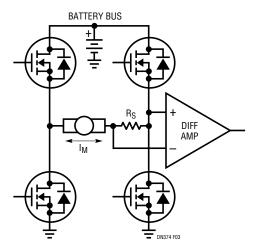
Many of the newer electric drive functions, such as steering assist, are bidirectional in nature. These functions are generally driven by H-bridge MOSFET arrays using pulsewidth-modulation (PWM) methods to vary the commanded torque. In these systems, there are two main purposes for current monitoring. One is to monitor the current in the load, to track its performance against the desired command (i.e., closed-loop servo law), and another is for fault detection and protection features.
