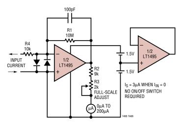
A floating amplifier circuit converts a full-scale 200nA flowing in the direction indicated at the inputs to 2V at the output of the LT1495. This voltage is converted to a current to drive a 200 $\mu$ A meter movement. By floating the power to the circuit with batteries, any voltage potential at the inputs are handled. The LT1495 is a micropower op amp so the quiescent current drain from the batteries is very low and thus no on/off switch is required.
