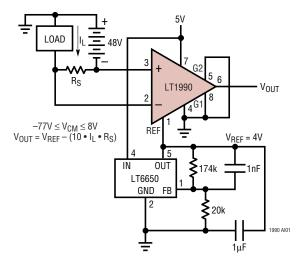
The LT1990 is a wide common-mode range difference amplifier used here to amplify the sense resistor drop by 10. To provide the desired input range when using a single 5V supply, the reference potential is set to approximately 4V by the LT6650. The output signal moves downward from the reference potential in this connection so that a large output swing can be accommodated.
