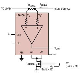
Instead of having fixed gains of 10, 12.5, 20, 25, 40, and 50, this circuit allows selecting between two gain settings. An NMOSFET switch is placed between the two gain-setting terminals (A2, A4) and ground to provide selection of gain = 10 or gain = 50, depending on the state of the gate drive. This provides a wider current measurement range than otherwise possible with just a single sense resistor.
