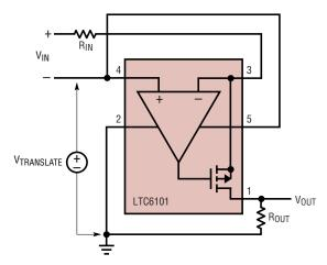
This is a convenient usage of the LTC6101 current sense amplifier as a high voltage level translator. Differential voltage signals riding on top of a high common mode voltage (up to 105V with the LTC6101HV) get converted to a current, through  $R_{IN}$ , and then scaled down to a ground referenced voltage across  $R_{OUT}$ .
