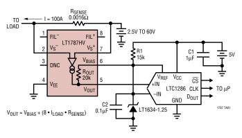
While the LT1787 is able to provide a bidirectional output, in this application the economical LTC1286 is used to digitize a unidirectional measurement. The LT1787 has a nominal gain of eight, providing a 1.25V full-scale output at approximately 100A of load current.
