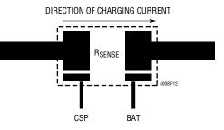
In any high current, >1Amp, application, Kelvin contacts to the sense resistor are important to maintain accuracy. This simple illustration from a battery charger application shows two voltage-sensing traces added to the pads of the current sense resistor. If the voltage is sensed with high impedance amplifier inputs, no IxR voltage drop errors are developed.
