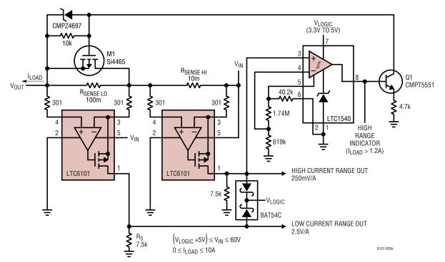
Using two current sense amplifiers with two values of sense resistors is an easy method of sensing current over a wide range. In this circuit the sensitivity and resolution of measurement is 10 times greater with low cur-
