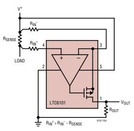
The second input resistor decreases input error due caused by the input bias current. For smaller values of  $R_{\rm IN}$  this may not be a significant consideration.
