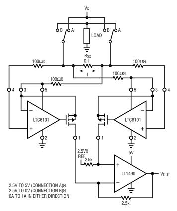
Two LTC6101's are used to monitor the current in a load in either direction. Using a separate rail-to-rail op amp to combine the two outputs provides a single ended output. With zero current flowing the output sits at the reference potential, one-half the supply voltage for maximum output swing or 2.5V as shown. With power supplied to the load through connection A the output will move positive between 2.5V and Vcc. With connection B the output moves down between 2.5V and OV.
