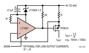
This is a simple current-source configuration where the op amp servos to establish a match between the drop on the sense resistor and that of the 1.2V reference. This particular op amp includes a shutdown feature so the current source function can be switched off with a logic command. The  $2k\Omega$  pull-up resistor assures the output MOSFET is off when the op amp is in shutdown mode.
