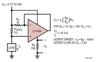
This circuit takes advantage of the microampere supply current and Rail-to-Rail input of the LT1494. The circuit is simple because the supply draw is essentially equal to the load current developed through  $R_A$ . This supply current is simply passed through  $R_B$  to form an output voltage that is appropriately amplified.
