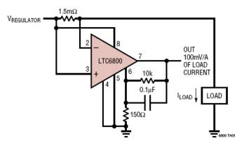
The low offset error of the LTC6800 allows for unusually low sense resistance while retaining accuracy.
