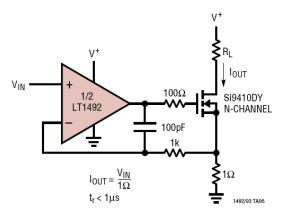
This is a simple controlled current sink, where the op amp drives the NMOSFET gate to develop a match between the  $1\Omega$  sense resistor drop and the  $V_{\rm IN}$  current command. Since the common-mode voltage seen by the op amp is near ground potential, a "single-supply" or Rail-to-Rail type is required in this application.
