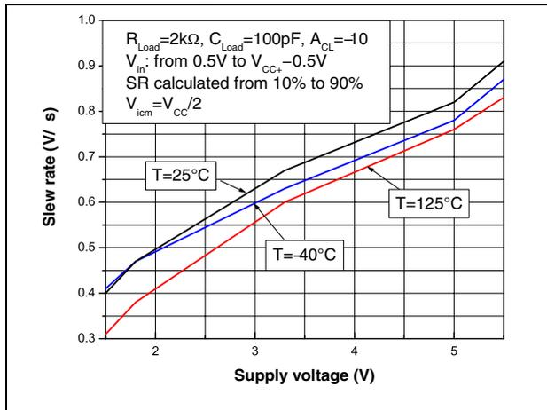
Figure 8. Negative slew rate vs. supply voltage
