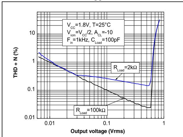
Figure 10. Distortion + noise vs. output voltage at V<sub>CC</sub> = 5 V
