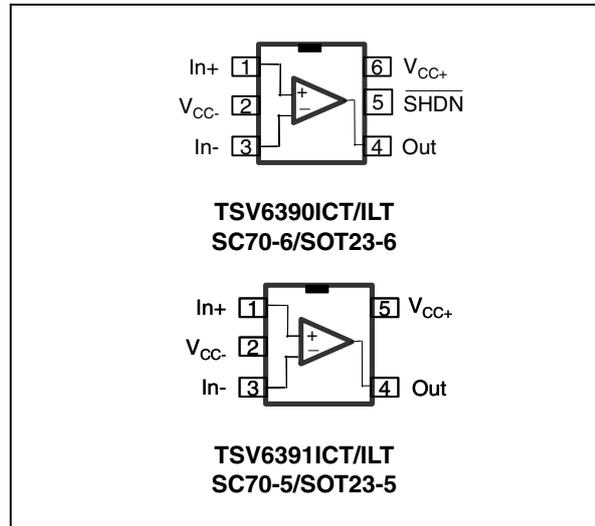
When used with a gain (above -3 or +4), these products feature an excellent speed/power consumption ratio, offering a 2.4 MHz gain bandwidth product while consuming only 60  $\mu$ A at a 5 V supply voltage.
