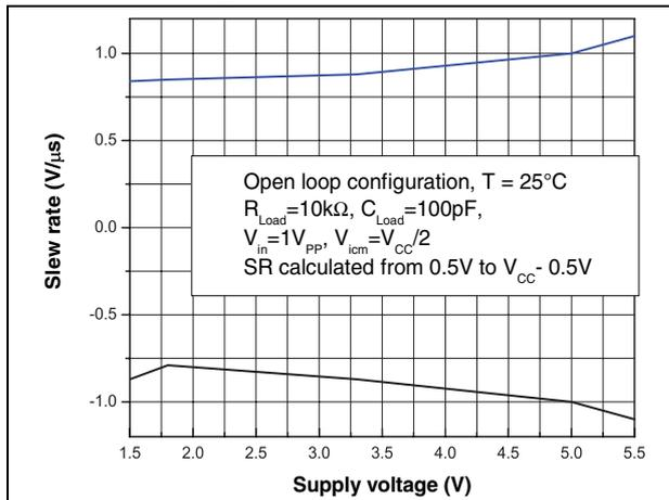
Figure 11. Slew rate timing in open loop
