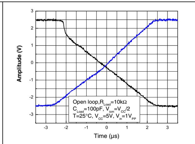
Figure 12. Slew rate timing in closed loop
