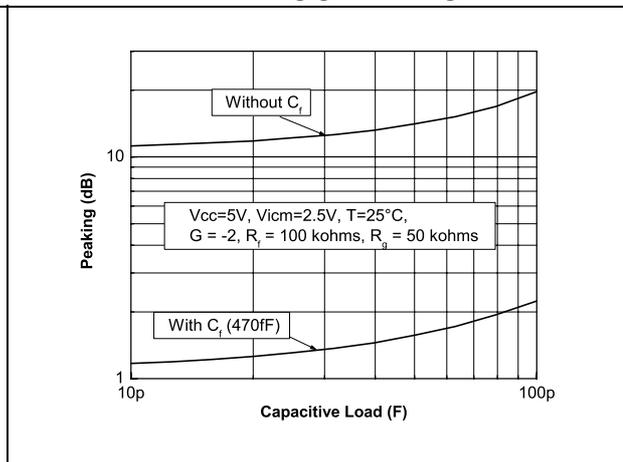
Another way to improve stability and reduce peaking is to add a capacitor in parallel with the feedback resistor. As shown in *Figure 16*, the feedback capacitor drastically reduces the peaking versus capacitive load (inverting gain configuration, gain = -2).
