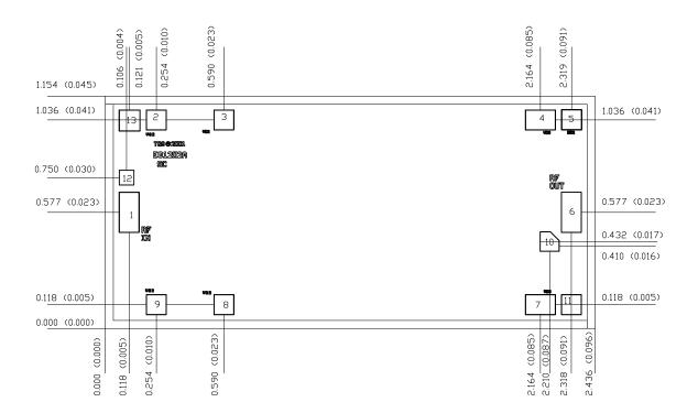
Units: millimeters (inches) Thickness: 0.100 (0.004)
