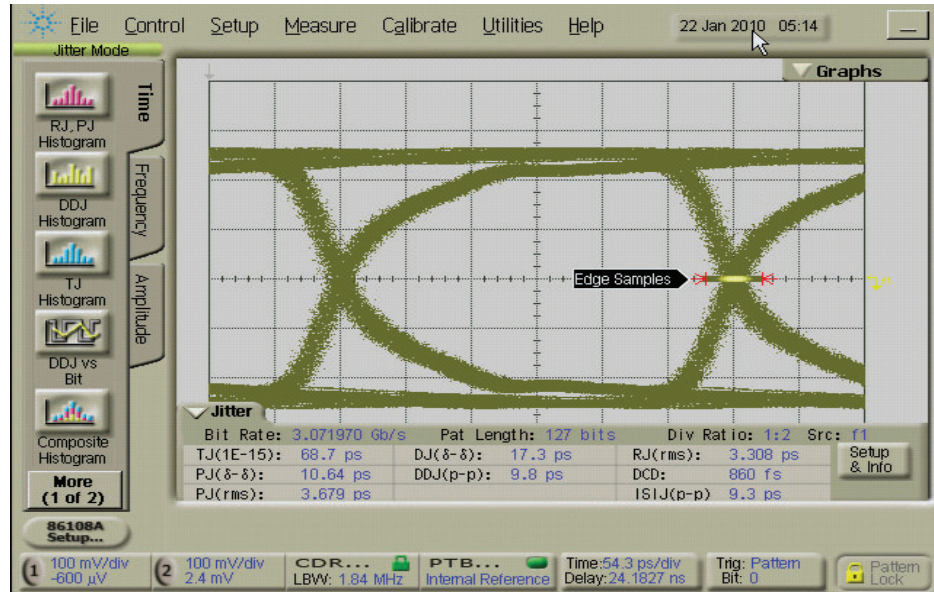
Figure 4: Transmitter Near-End Output Eye (3.072 Gb/s)
