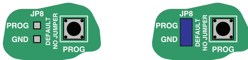
a) No Jumper: FPGA Operational (default)
